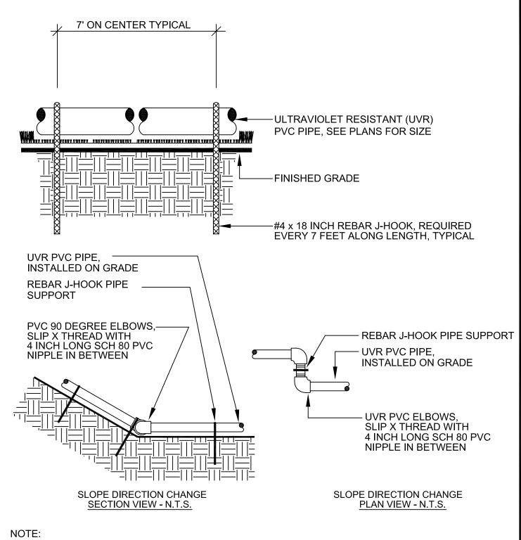
ALL PVC PIPE AND FITTINGS INSTALLED ON GRADE TO BE ULTRAVIOLET RESISTANT (UVR). USE TEFLON TAPE ON THREADED FITTINGS.
