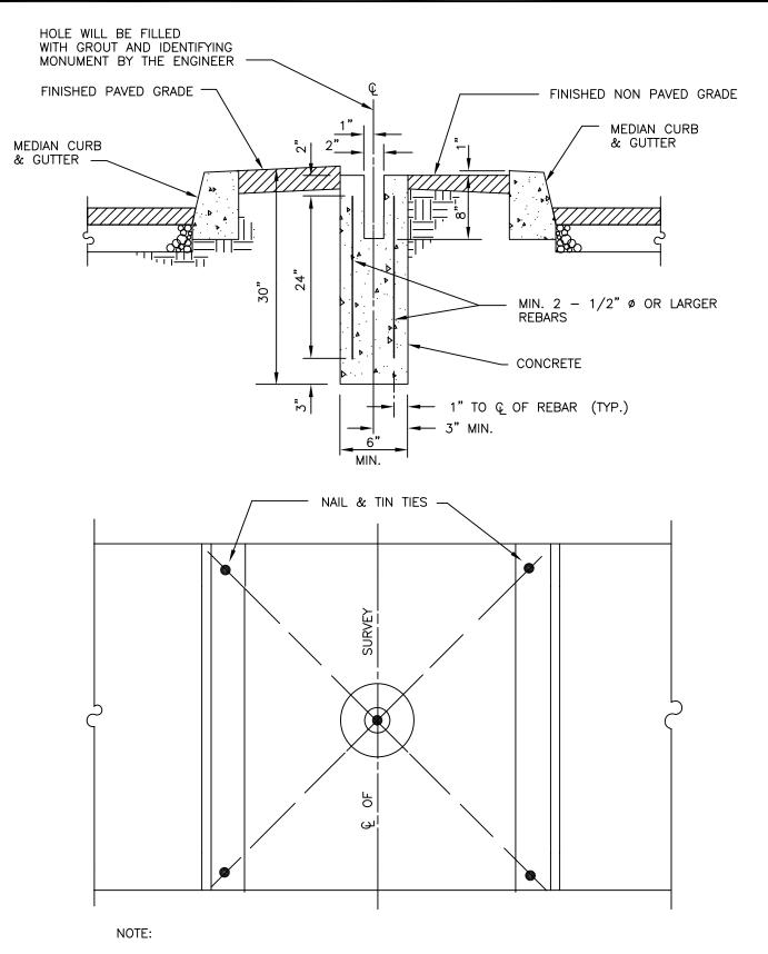
1. THIS TYPE OF MARKER TO BE INSTALLED ONLY IN RAISED MEDIANS.
